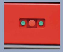
At the vehicle left rear side, there are the operating switches (front and behind electric switches, emergency power shut-off switch). The hook can be conveniently and safely manipulated
