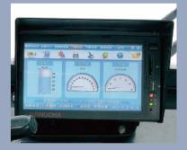
Remote control (optional): Vehicle management system: Vehicle status enquiry and record, alarm for overspeed, door lock, radar and so on. The equipment can be provided with 7-inch touch screen. The operation is simple and convenient. With overall data display & real-time status reminding, monitoring, management and service can be realized in remote way
