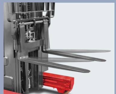
Forks can tilt forward/backward for easy loading
