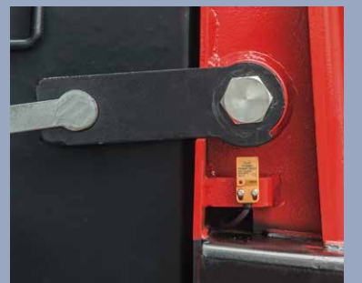
The locking device of the battery is provided with the safety protection function. Only if the locking device is rotated in place, the tractor can travel
