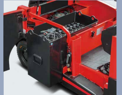
Battery side roll out is taken as the standard configuration in order to easily and fast replace the battery
