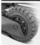
The front wheels are equipped with deep groove rubber tires. with large ground clearance, wear resistance and durability, and good shock absorption
