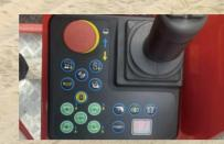
Portable drive box integrates drive and lift and one button leveling function, The steering control is arranged at the end of the handle, so that the single handle can flexibly control the travelling speed, steering function and lifting height of fence.
