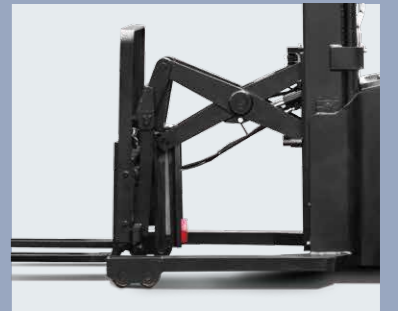
Forks move forward by the scissor structure
