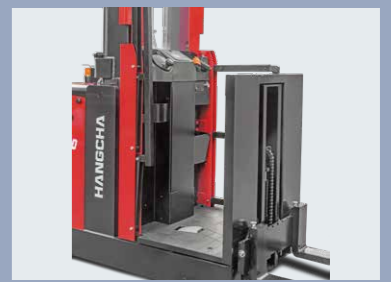
Order picker works only when the side barriers are all lowered
