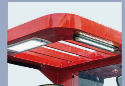
LED top lamp can provide bright operating environment
